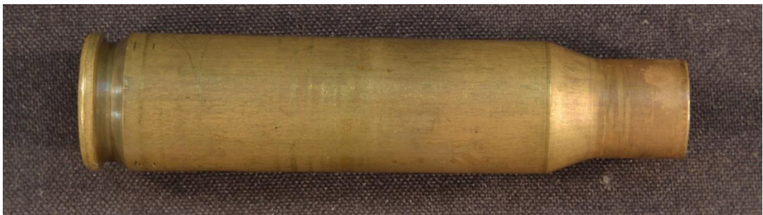
Figure 2 – 0.308 Lapua cartridge case after 5 firings
