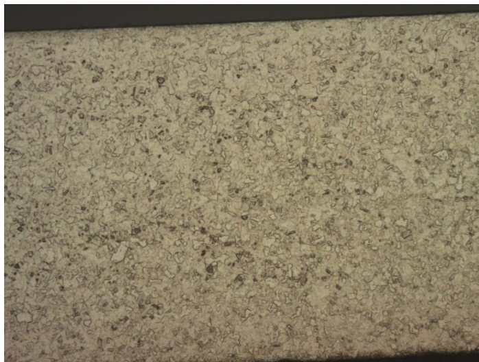
Figure 19 – Neck microstructure; Stage 11; sample set C (200 times magnification)
