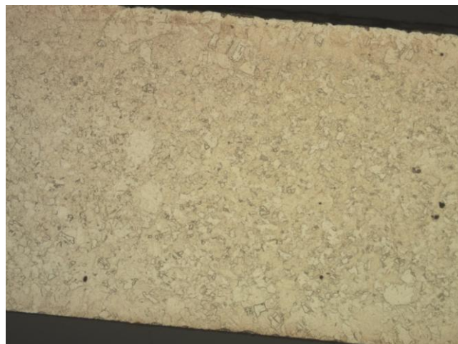
Figure 21 – Neck microstructure; Stage 7; sample set BAA (200 times magnification) Cartridge BAA-7-1 LHS of neck
