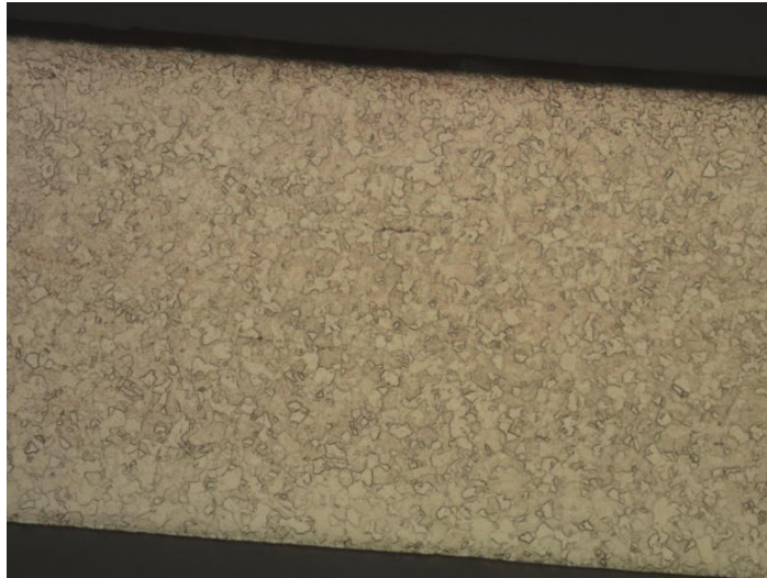
Figure 17 – Neck microstructure; Stage 0 (factory) (200 times magnification)
