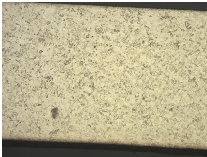
Figure 18 – Neck microstructure; Stage 11; sample set A (200 times magnification)
