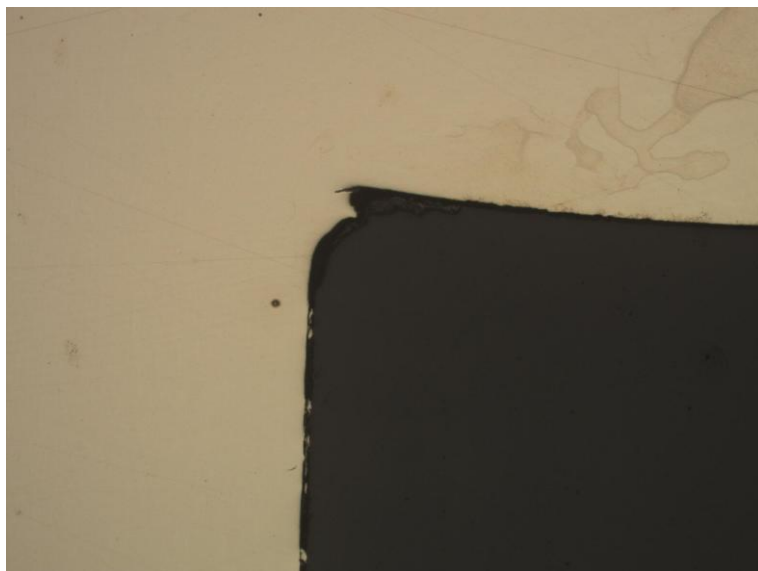
Figure 10 – Crack at inside corner of primer pocket in sample A-6-1 (50 times magnification) Cartridge in vertical position
